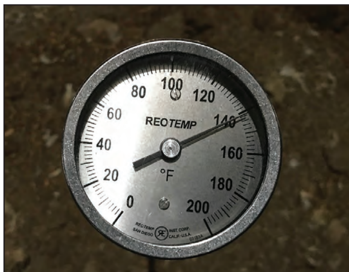
Figure 3. Use a compost thermometer to check litter temperature.
